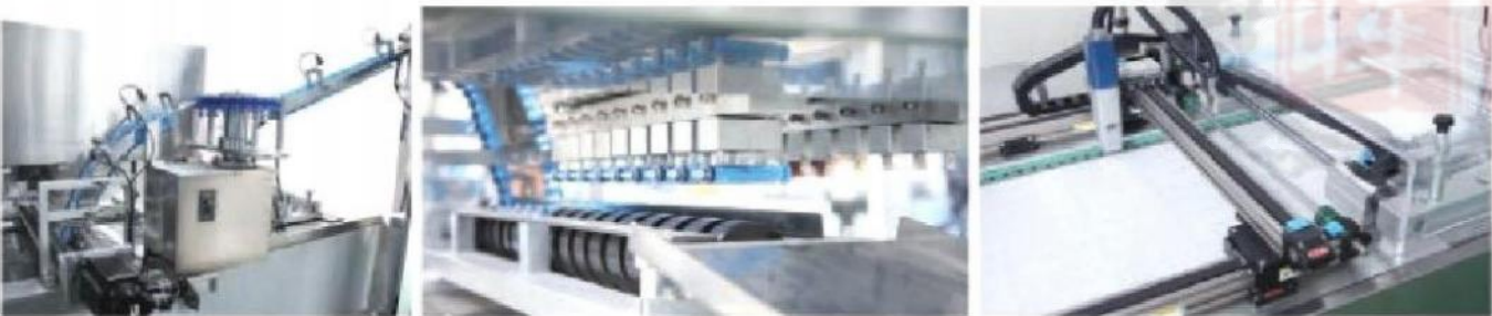
▲ Mechanical hand automatic feeding ▲ No needle rejection device ▲ Ink jet printing with X,Y direction
